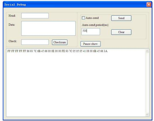
In this interface, click "Auto-send" or "Send" will combine data head, data, and check code into one frame and send out it. The data that the gateway received from HART fieldbus will be shown in the blank place below.
