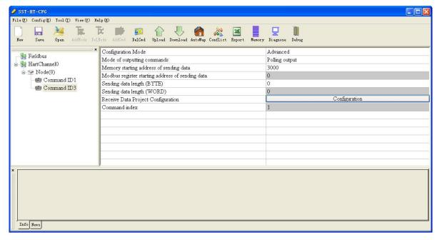
This interface details is described in chapter 4.2.4.4, so here we don't describe it. The below is the example of No.3 HART command, to show how to use "Segment Mapping" function, we can see one "configuration" button after the "receive data project configuration" option, click it:
