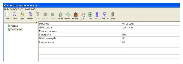
Note: HART protocol specifies that the slave device which address is 0 must work in single-point mode. In single-point mode the digital communication and analog communication is allowed to exist at the same time. The Slave with address 1~15 works in multi-point mode. In multi-point mode the analog output of the device is the minimum value (e.g. 4mA), only allows digital communication. The protocol also specifies that the default factory address of field device is 0.
