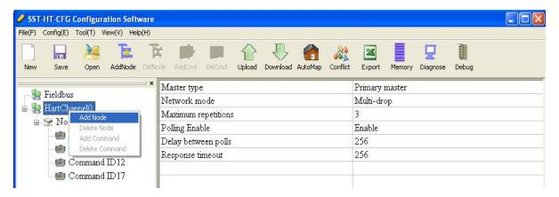
Click the added node, set slave address in the right configuration plate, and please notice that HART channel can only be equipped with one slave node when configured in the single point mode.
