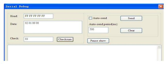
In this example, command ID0 is composed of data head, data and check code. It uses short address; when you click "Send", you will get the response data.
