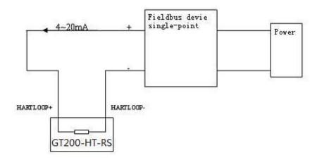
Using the internal resistor!
