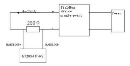
Not using the internal resistor!
