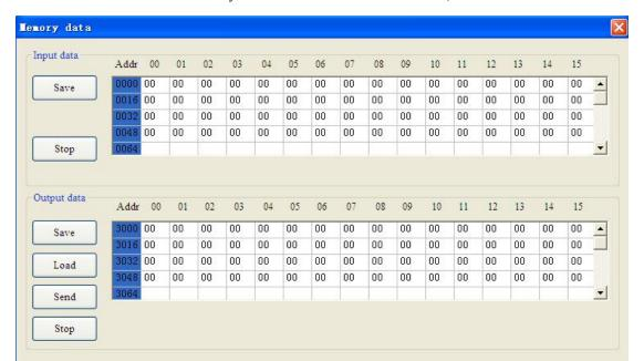
As is shown in the table, upper table shows the memory distribution of HART input data, lower table shows the output data. When you need to change the output data, click the "stop" button firstly, then change the related data or load the already saved data table, at last, click the "sending data".
