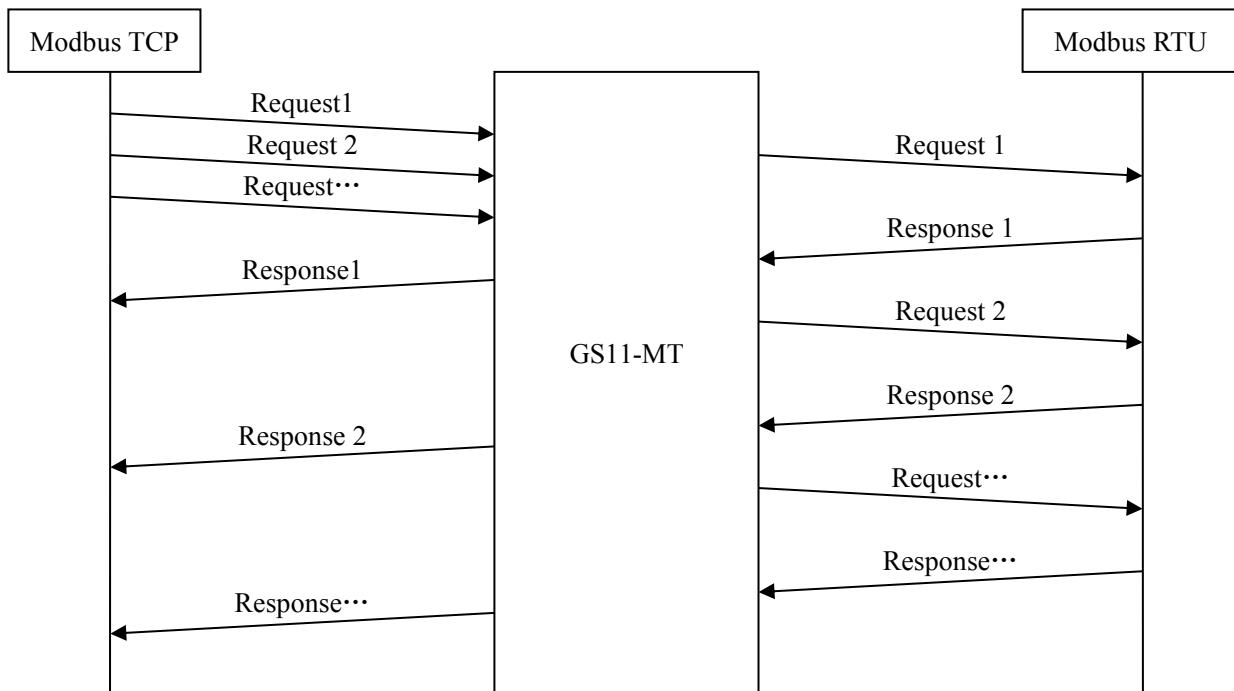
Every Modbus TCP can connect multiple requests at the same time in this mode, and all connections share the request buffer which can cache 20 frames.
