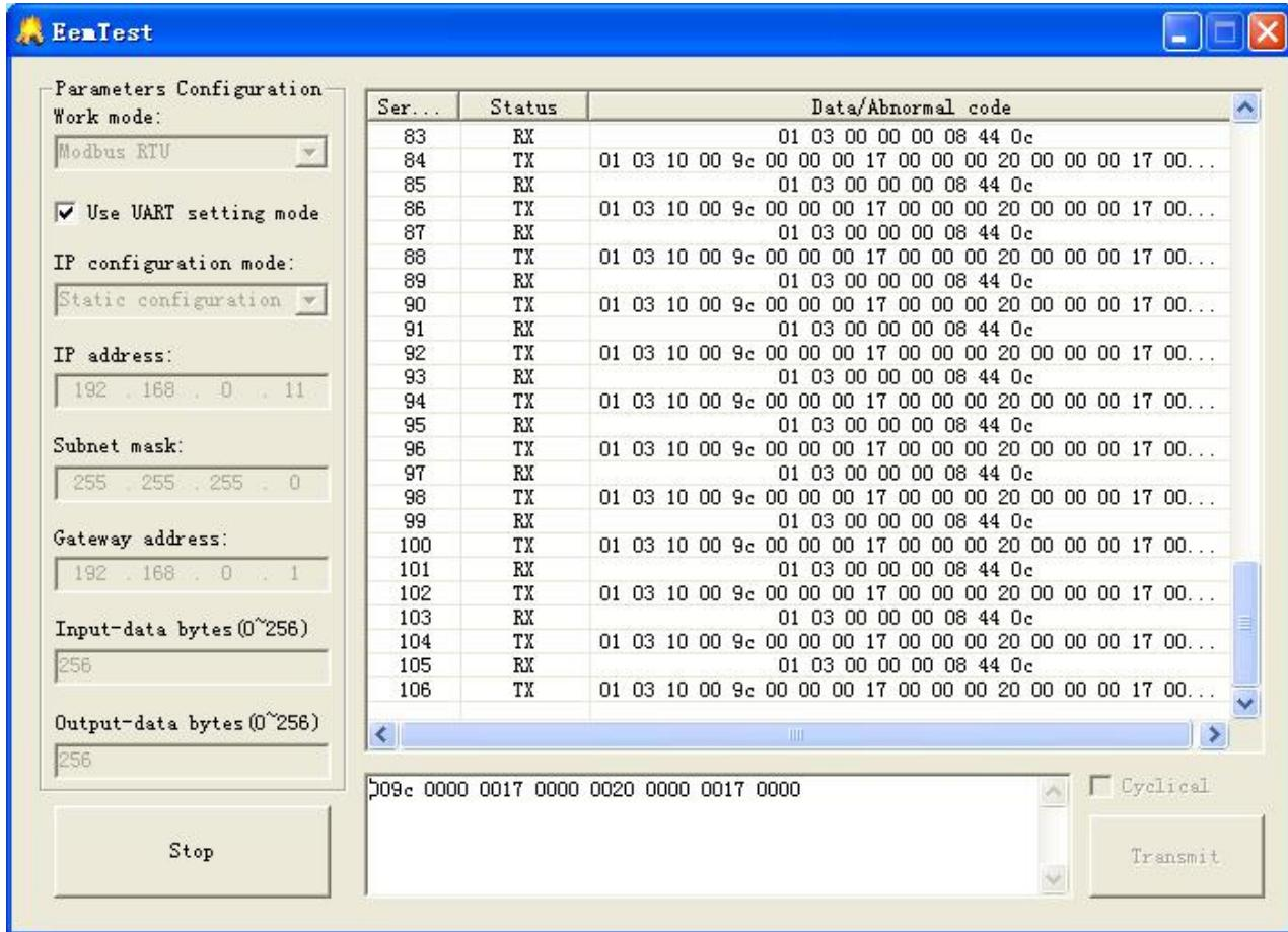
**Note:** RX is the data received, TX is the data transmitted.
