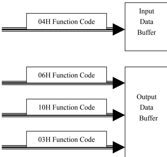
04H function code is used to read input data; 06H and 10H function codes are used to write output data; 03H function code is used to read back output data, and then multiple Modbus TCP masters can exchange data using this function code.
