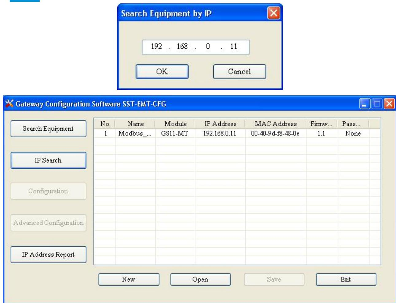
After entering the wanted IP address, click OK, the software will search GS11-MT with the named IP address in the network, and list the information of the equipment in the table.
