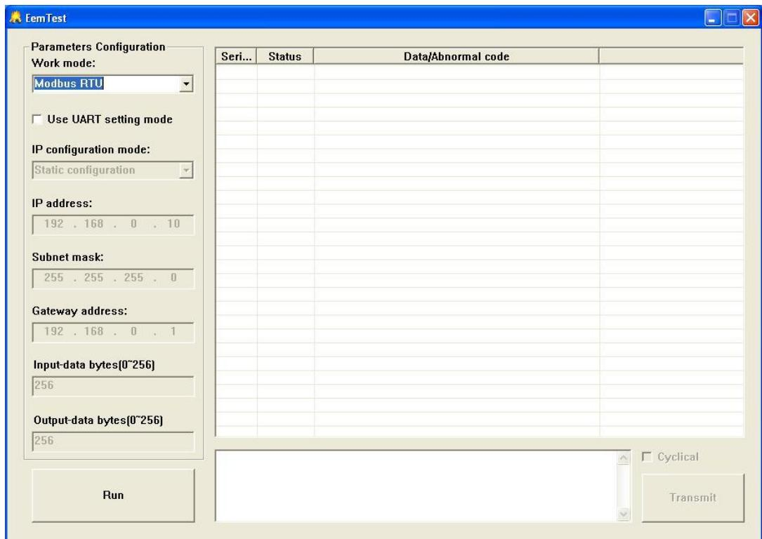
SST Automation-defined protocol work mode: test software is the communication initiator, and the module responses. The interface is as follows:
