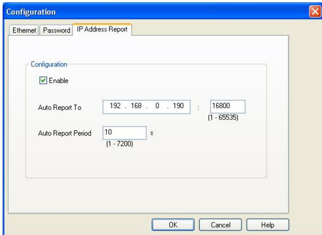
Select the check box before the “Enable”, the parameters can be configured:
