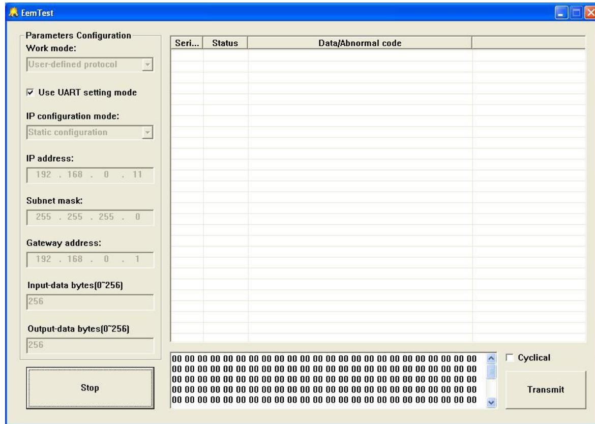
If the connection is failed, there will pop up an alert dialog, and the options in the Parameters Configuration section will not be grayed.
