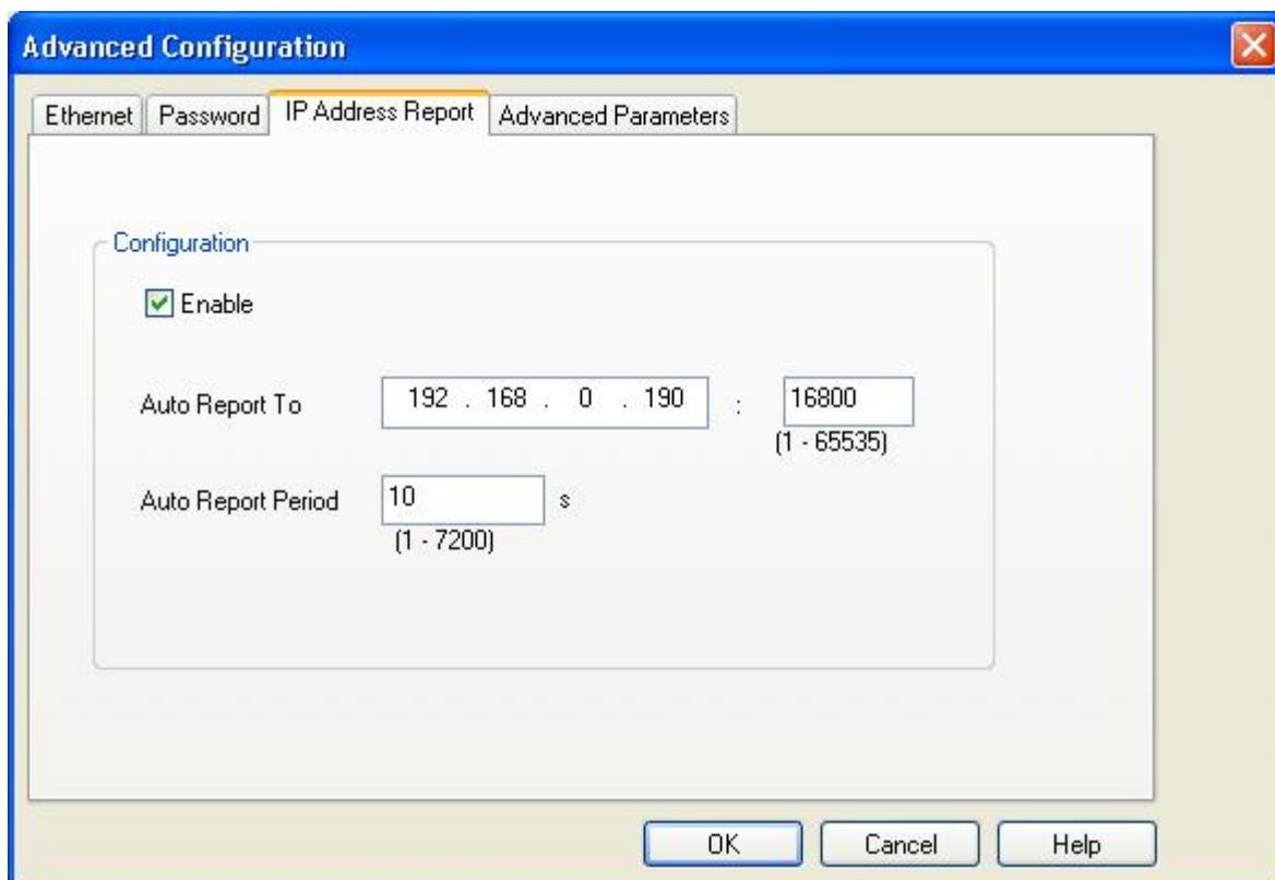
Select check box before the “Enable” , the parameters can be configured:
