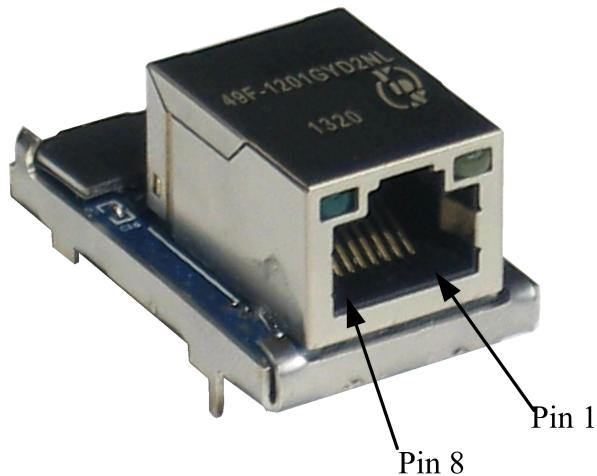
The Ethernet interface uses an 8-line RJ-45 interface, and the pin definitions are as follows:
