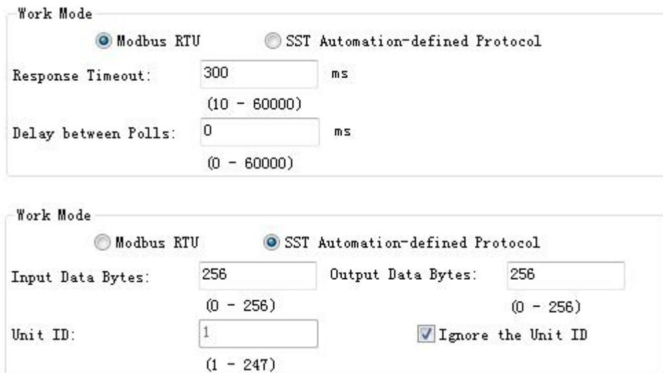
In “SST Automation-defined protocol” mode, you need to set “Input Data Bytes”, “Output Data Bytes” and “Unit ID”.
