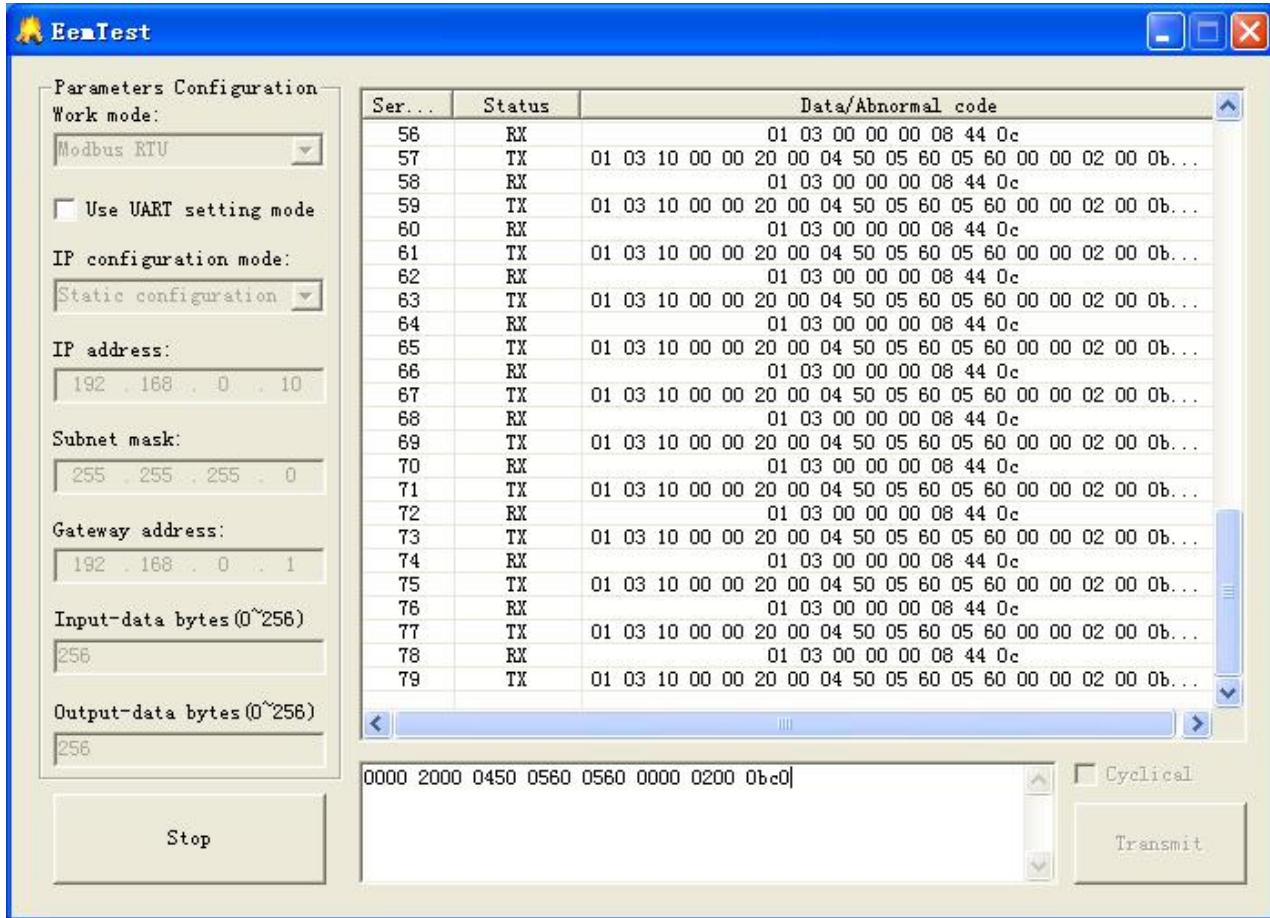
Transmit data: After establishing connection successfully, software receives data, and transmits data according to Modbus protocol and displays them. Testing software currently only supports 03H and 10H function codes (GS11-MT supports all the Modbus function codes, and supports the maximum data length allowed by the protocol.), and 8 registers, and the start address of the register is 0(40001), users only need to modify the relevant data in the data transmitting section.
