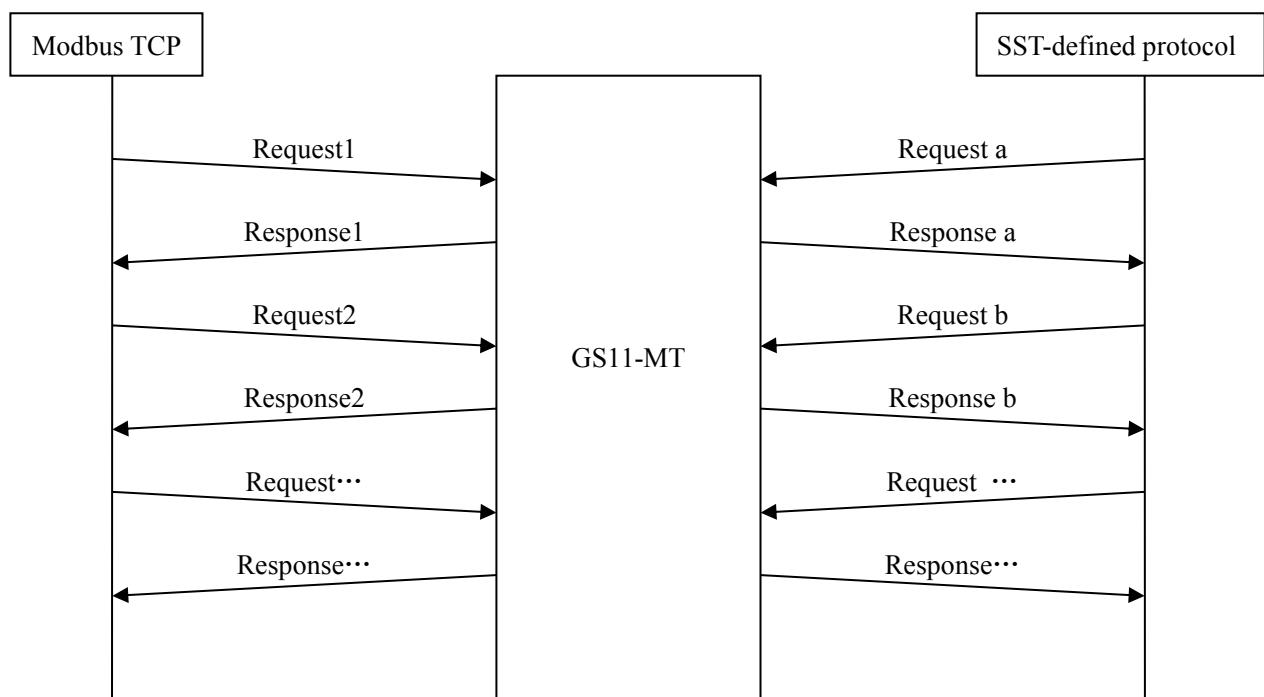
In this mode, Modbus TCP only supports 03H、04H、06H、10H function codes.
