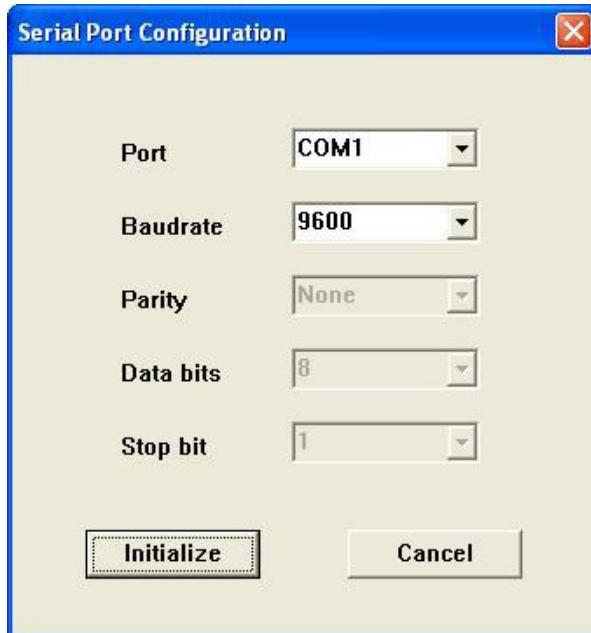
“Port” is the serial port being used; “Baudrate” is current serial port baud rate set by DIP switches.
