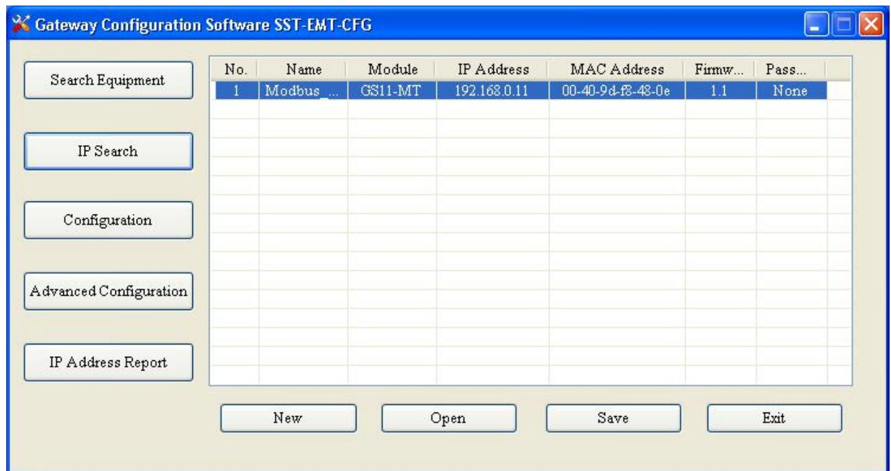
Click “Advanced Configuration” button, a password dialog box will pop up if the equipment has been set up with a password; The Advanced Configuration window will appear when your entering password is correct.
