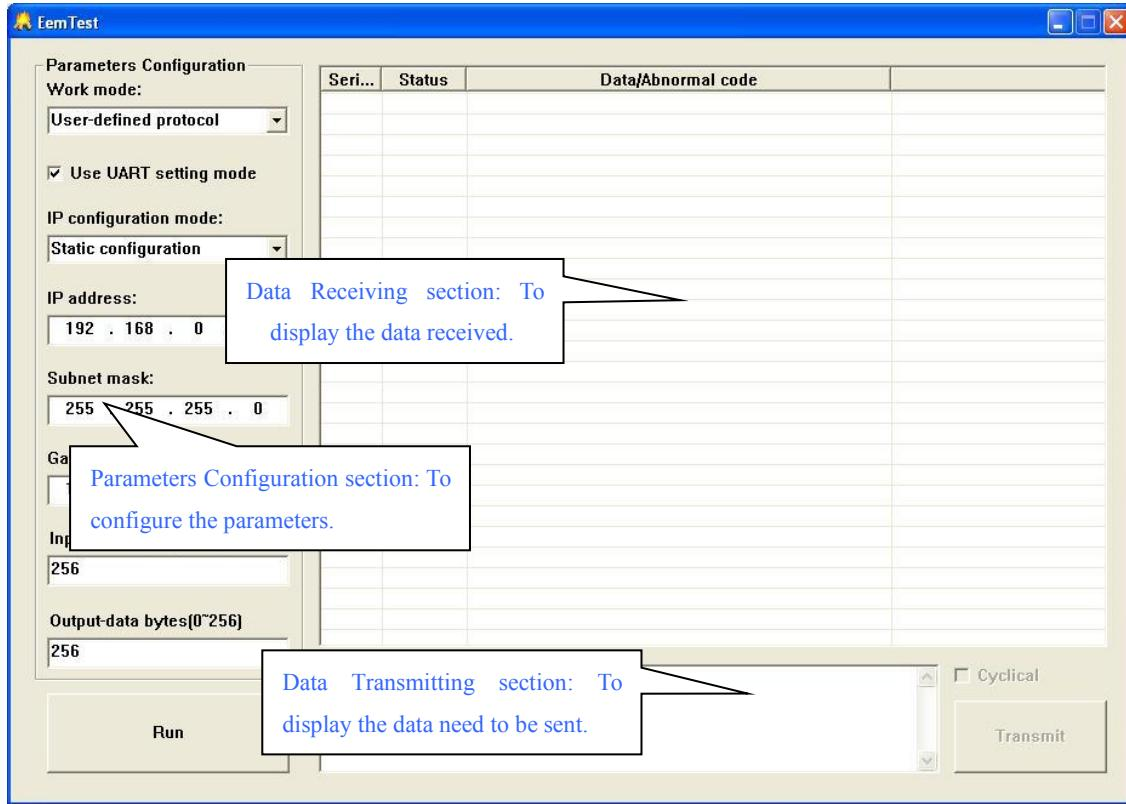
Work mode: The first combo box in Parameters Configuration session is to set work mode.
