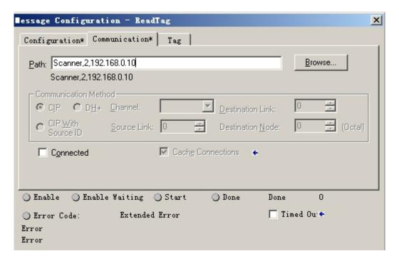
Add a "MSG" command in "MainRoutine" under the "MainProgram" and choose "ReadTag" as "Message Control", as shown below:
