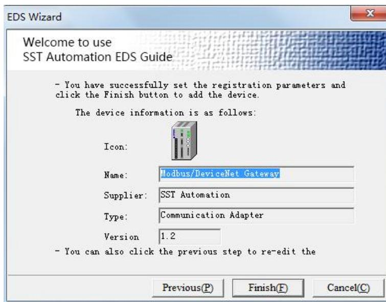
Click "Finish" and the EDS file registration step is over. At this time, you can see the newly registered device in the equipment Management Window.
