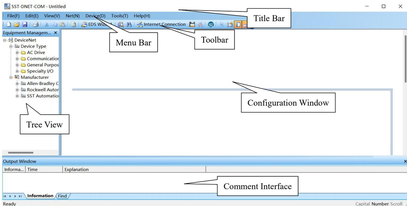
**Configuration window:** After establishing the internet connection, display the online device and modify the address and parameters of the device online, check the input and output data. In the offline state, you can view device properties by dragging the device icon to the window.
