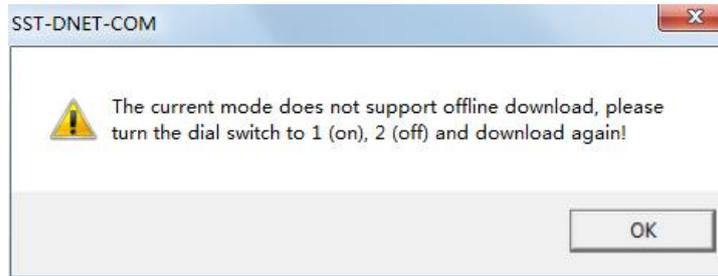
About 5s after the DIP switch is set to 1ON 2OFF, the device can download configuration. After downloading, it will prompt that the download is successful and the downloaded configuration will take effect after restarting the device, and it will prompt that the DIP switch should be set back to 1OFF 2OFF.
