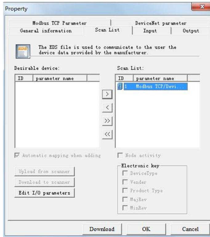
Add adapter station 9 to the scanner station mapping list, and then select adapter station 9 in the "Scan List". After selecting it, click "Edit I / O parameters". This interface sets the number of input and output bytes of the adapter:
