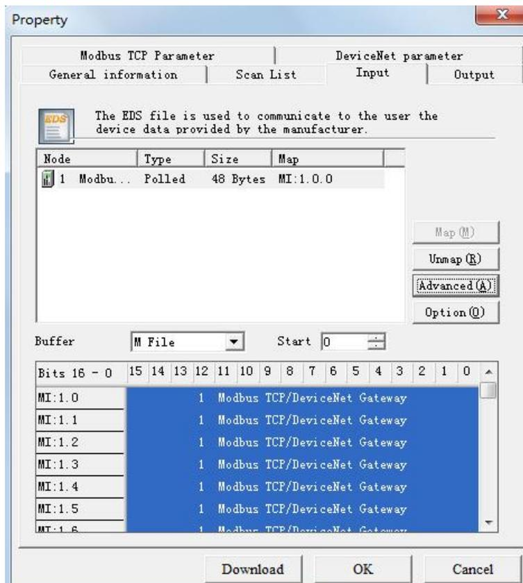
If you need to set the unit that maps the starting address in "advanced I/O mapping Settings", click "option" button to set it. As shown in the figure below, "Byte Align" means in one byte and "Word Align" means in two bytes:
