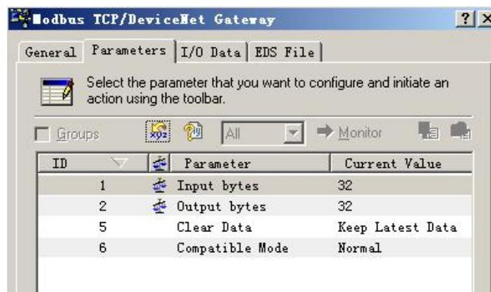
Input Bytes: DeviceNet I/O connection input bytes.
