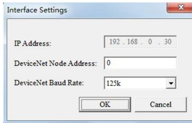
Notes: the interface settings configuration, "IP address" is the IP of the device selected at the time of search. "DeviceNet Node Address" is the Address of DeviceNet Scanner Module. Set any value between 0 and 63, which can't conflict with other node addresses on the bus. "DeviceNet baud rate" is the baud rate of DeviceNet scanner module, 125K, 250K, 500K optional. Keep Bus Baud Rate Consistent.
