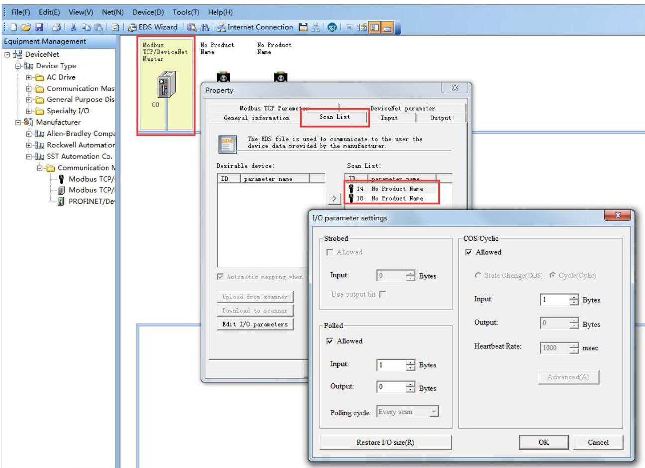
The modified configuration parameters can be downloaded to GT200-MT-DN. GT200-MT-DN as the DeviceNet
