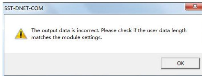
Note that after the address is changed in the general interface, because the device with the modified address will be restarted and the DeviceNet internet connection has been disconnected, at this time, the I/O data input and output operation will not be able to see the data, You need to disconnect SST-DNET-COM's "Internet Connection" and re-establish the internet connection.
