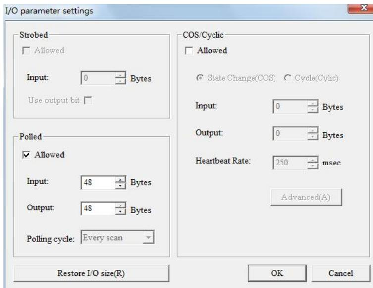
Notes: If the I/O parameters of the node have been saved in GT200-MT-DN, the scanned I/O parameters are the saved I/O parameters. if the I/O parameters of the node have not been saved in GT200-MT-DN, this I/O parameter is the default value, and users can configure it according to the actual I/O parameters.
